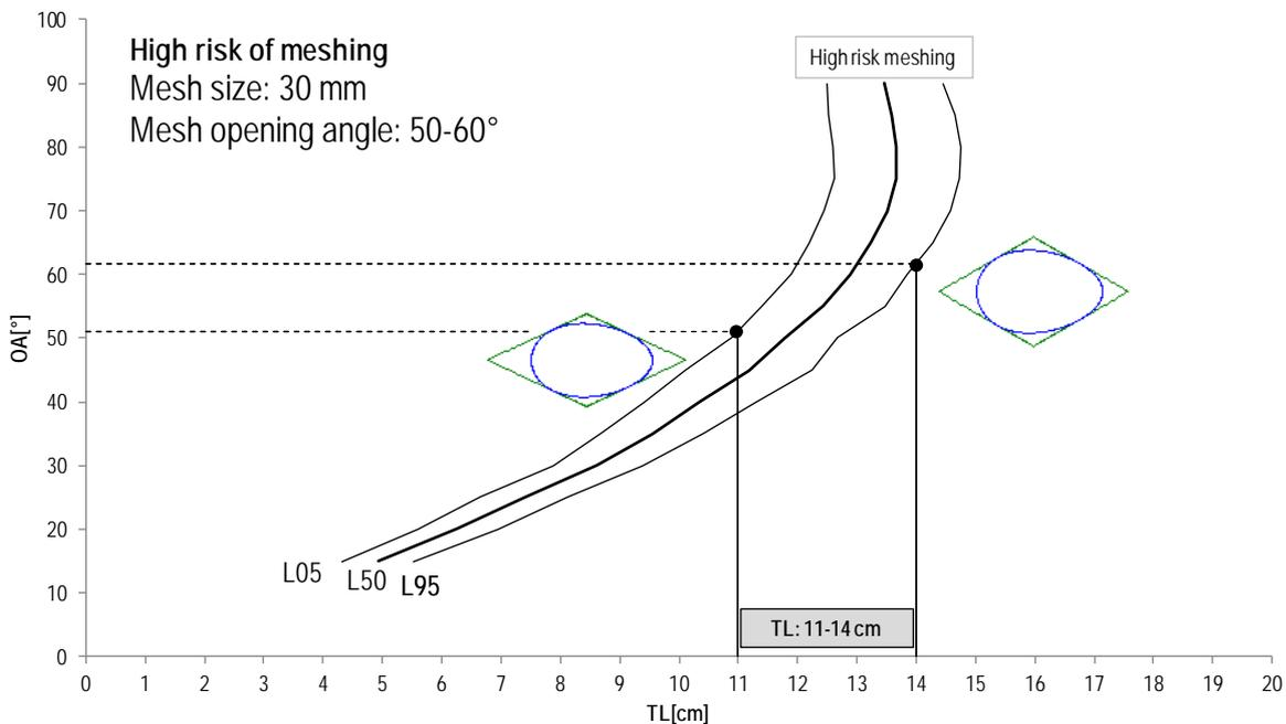
Figure 73. FISHSELECT analysis of risk of meshing for anchovies. L05, L50 and L95: retention length at 5, 50 and 95 %; OA: mesh opening angle; TL: total fish length.
