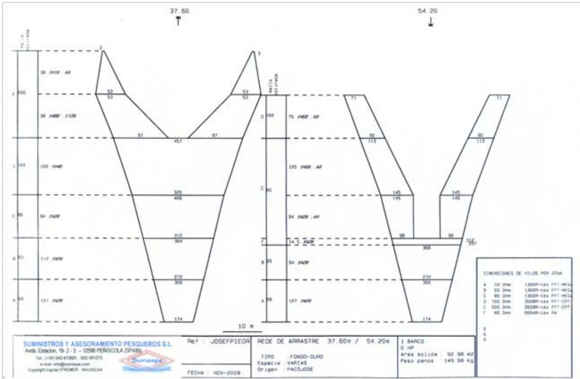
Figure 42. Schematic diagram of the commercial bottom trawl net used on the shallow shelf fishing grounds during the short pilot action developed off Menorca (Balearic Islands, western Mediterranean).
