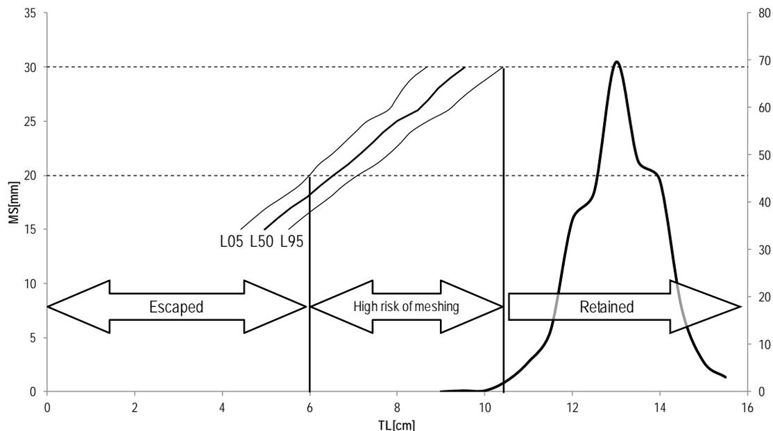
Figure 74. FISHSELECT analysis of risk of meshing for anchovies compared to fished anchovy population (thick curve). L05, L50 and L95: retention length at 5, 50 and 95 %; MS: mesh size; TL: total fish length.
