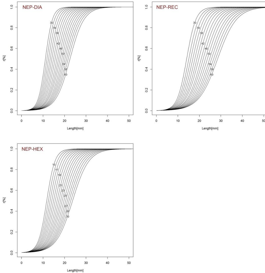
Figure 40. Selectivity guidelines with predicted selectivity of Norway lobster (*Nephrops norvegicus*) in different mesh sizes. Predictions are made from 30 to 60 mm meshes in steps of 1 mm assuming a similar distribution of mesh opening angle.
