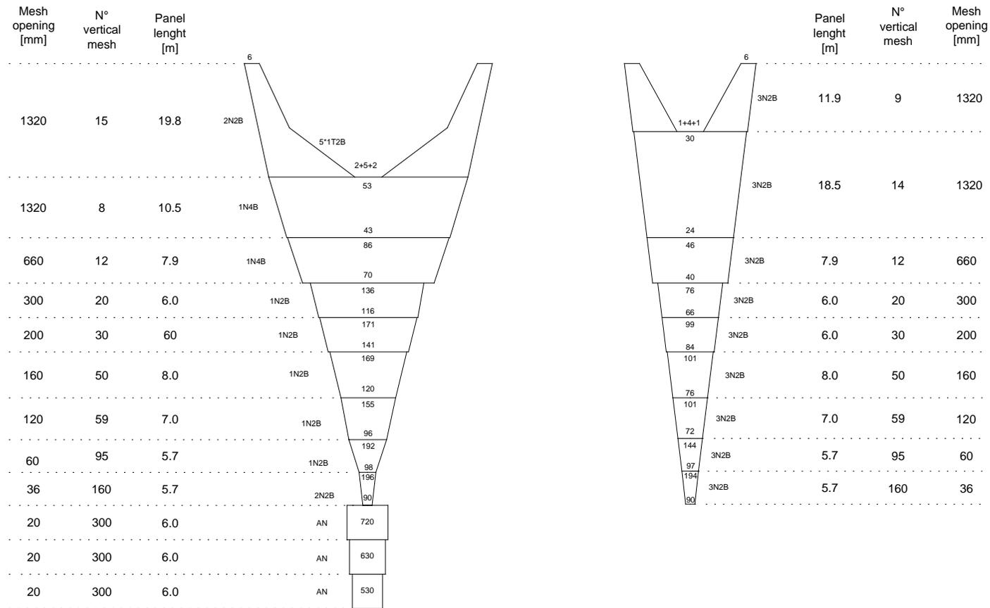
Figure 68. Original design of the single-boat pelagic trawl.
