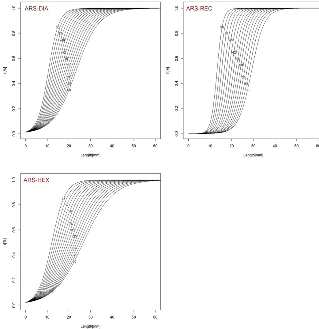
Figure 34. Selectivity guidelines with predicted selectivity of giant red shrimp (*Aristaeomorpha foliacea*) in different mesh sizes. Predictions are made from 30 to 60 mm meshes in steps of 1 mm assuming a similar distribution of mesh opening angle.
