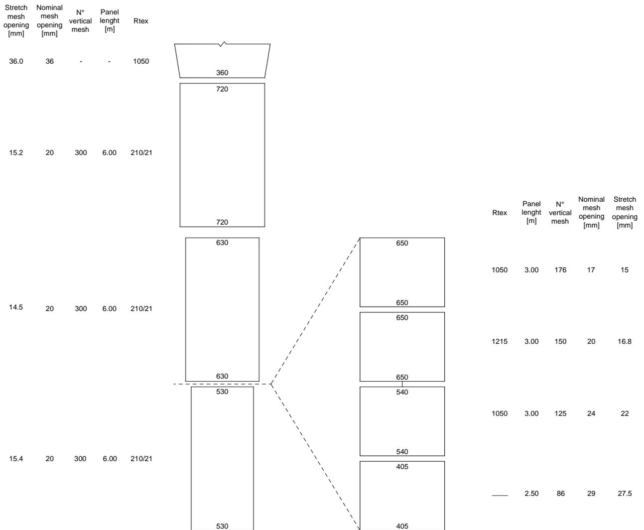
Figure 70. Design and technical specifications of the codend of the net. The four nettings on the right have been mounted before the last codend netting piece as showed by the dashed line.
