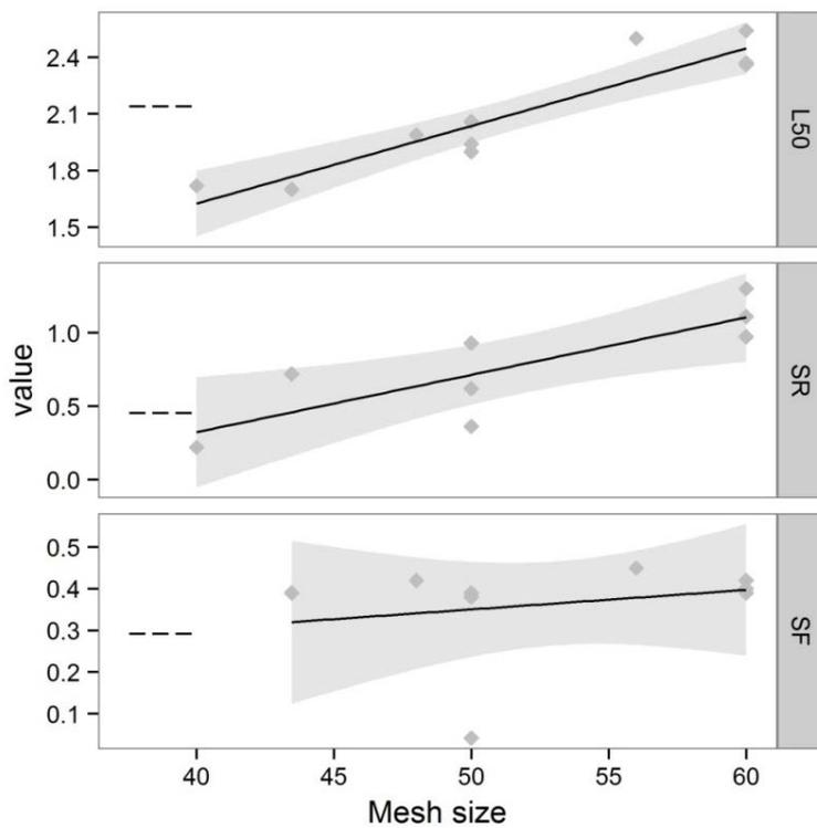
Figure 25. Relationship between selectivity parameters (L50% and SR) and mesh size for *A. antennatus*. Solid line represents DM codends, dashed line represents average value for SM codends.
