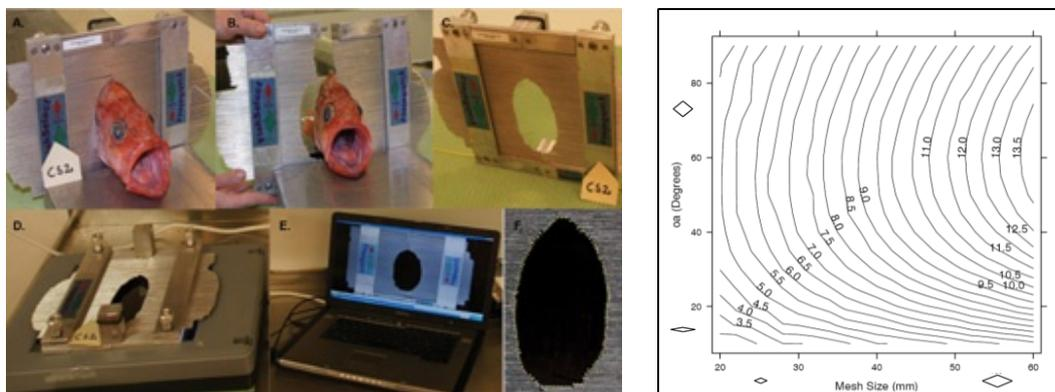
Figure 8. Fish being measured using FISHSELECT morphometer (left); example on Design Guide for diamond meshes for a specific species (right). It shows ISO curves for the size of fish that based on morphology would be able to escape through diamond meshes of different mesh size (X-axis) and different opening angle (Y-axis).
