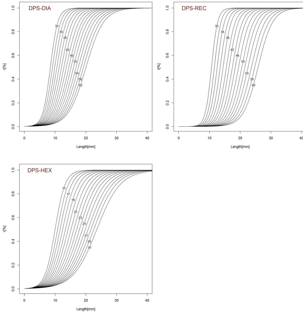
Figure 38. Selectivity guidelines with predicted selectivity of deep-water rose shrimp (*Parapenaeus longirostris*) in different mesh sizes. Predictions are made from 30 to 60 mm meshes in steps of 1 mm assuming a similar distribution of mesh opening angle.
