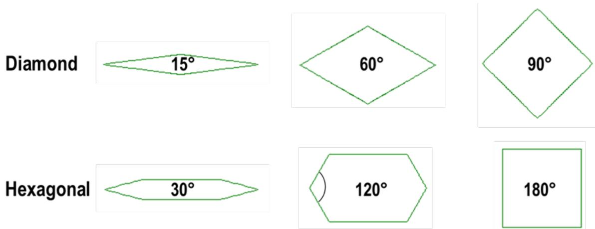
Figure 31. Illustration of the range of the mesh openings investigated both for diamond- and hexagonal-meshes for the guideline design of fish size-selective mesh.
