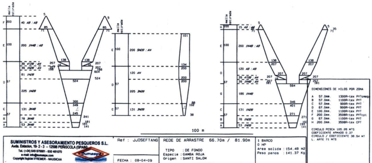
Figure 43. Schematic diagram of the commercial bottom trawl net used on the middle slope fishing grounds during the short pilot action developed off Menorca (Balearic Islands, western Mediterranean), within the framework of DISCATCH project.
