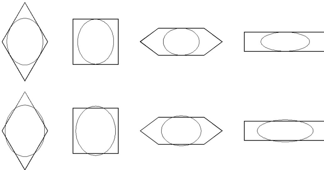
Figure 30. Mesh penetration process in stiffness condition without compression. Upper images represent the condition in which fish can pass through the meshes, the cross-section shape represented by the ellipse are at most of the same dimension of the mesh shape. The images below represent the condition in which the fish do not pass through the meshes, the cross-section shape are bigger than the mesh shape.
