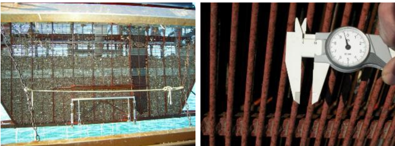
Figure 23. There are national laws that define some aspects of the capacity of the gear to select the size of the clams caught. The D.M. of 22/12/2000 states that the distance between the metal rods on the lower part of the dredge must not be less than 12 mm.
