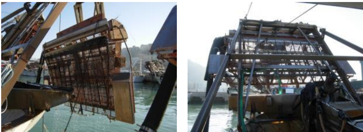
Figure 2. details of a hydraulic dredge.
