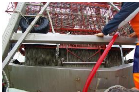
Figure 25. Detail of the dredge consisting of cage made entirely of metal (left). All clam dredgers have the dredge at the bow of the vessel; at the end of each dredging operation, the dredge is hauled on to the bow with the hauling warp and the material gathered is transferred into a collection box (right) and then to a sieve for the selection of the marketable sizes.
