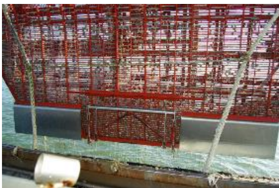
Figure 25. Detail of the dredge consisting of cage made entirely of metal (left). All clam dredgers have the dredge at the bow of the vessel; at the end of each dredging operation, the dredge is hauled on to the bow with the hauling warp and the material gathered is transferred into a collection box (right) and then to a sieve for the selection of the marketable sizes.
