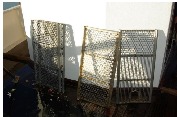
Figure 24. Detail of the vibrating sieves with a perforated metal grate, the holes must not be smaller than 21 mm.
