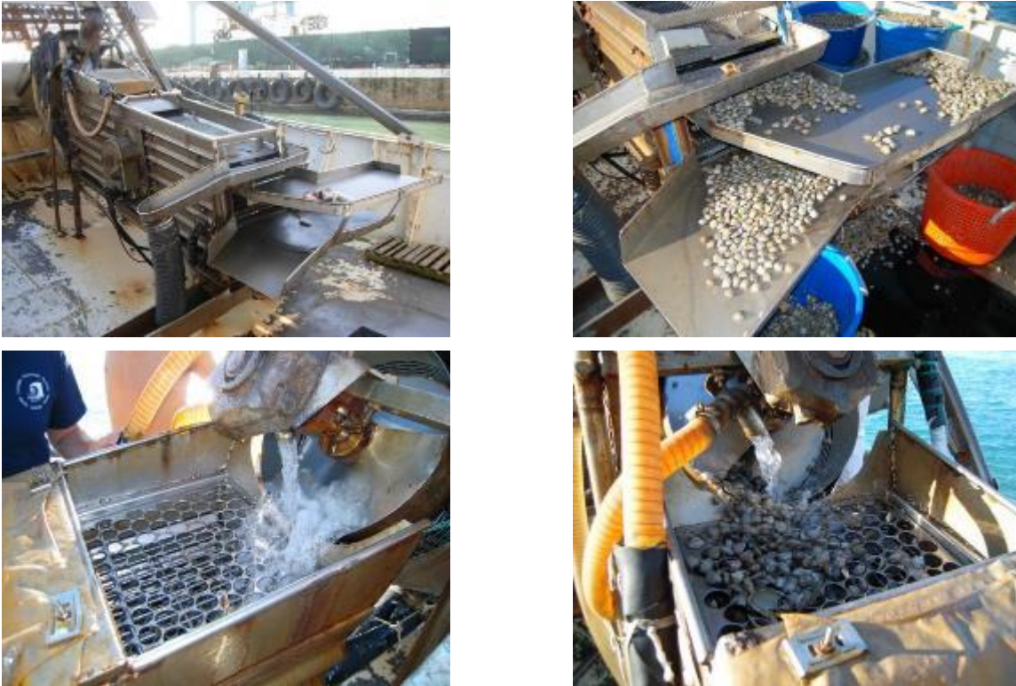
Figure 26. Details of the vibrating sieve used on board clam dredgers to select the clams of marketable sizes ( \geq 22 mm).
