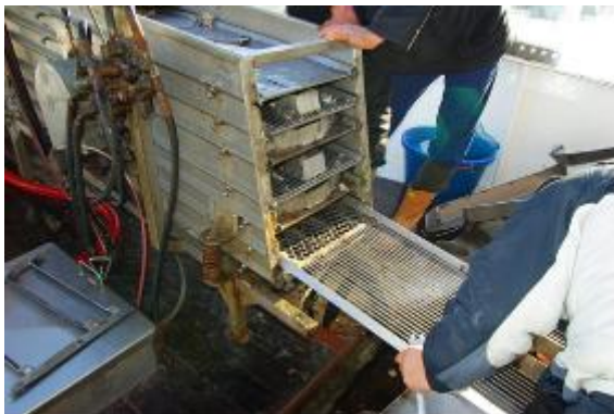
Figure 24. Detail of the vibrating sieves with a perforated metal grate, the holes must not be smaller than 21 mm.
