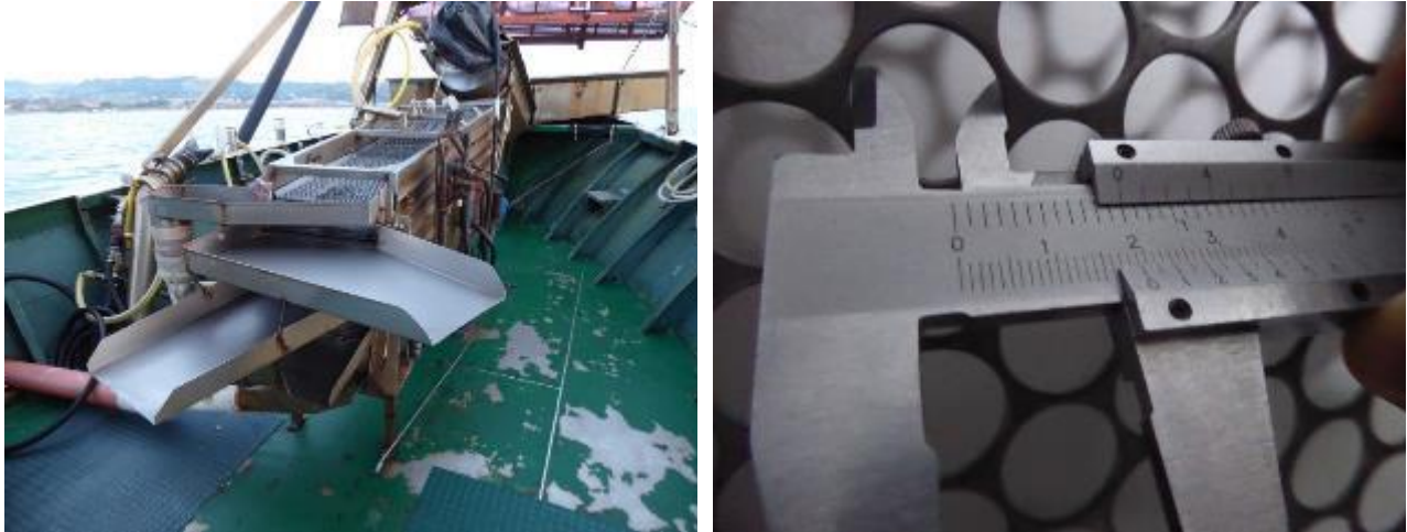
Figure 15. vibrating mechanical sieve used on board hydraulic dredgers to select the size classes of product that can be marketed, and the 19 mm grill used during the surveys (b).
