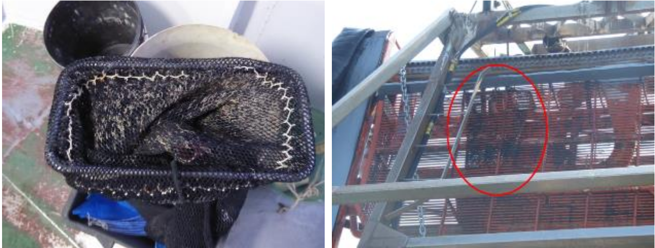
Figure 16. sampling net made of a stainless-steel frame (40 cm internal length, 20 cm internal width with a thickness of 1 cm) and a nylon net with 12 mm mesh.
