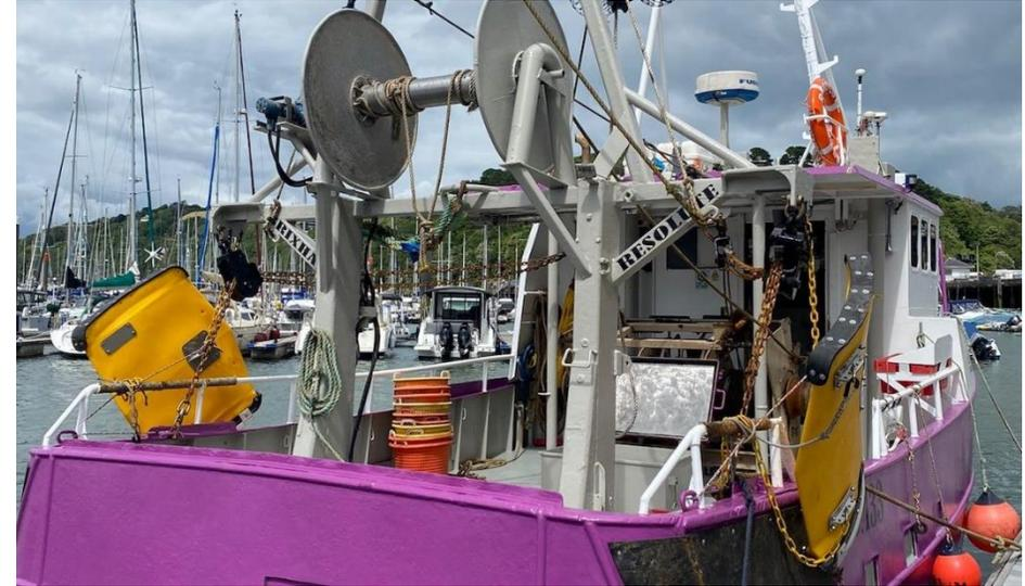
Trawl doors made partly from **recycled plastic** (weight 95kg), **reduction in fuel consumption** by as much as **30%**.
