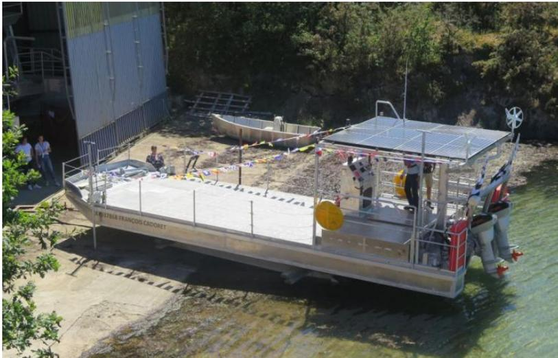
Two 70 kW electric motors with **two 40 kWh batteries** powered via **solar panels** and two small **wind turbines**. Later, it will be able to receive a **hydrogen kit**.
