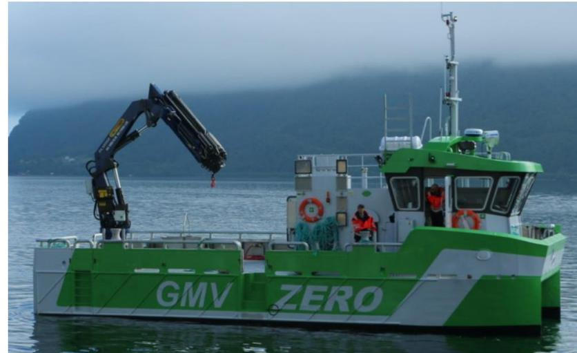
**Battery** power of **340 kWh**, **no emissions**, engine noise or fumes. Estimated **annual savings** are **80%** on maintenance costs, **33.700 litres** of diesel/year saved with **90 tons CO<sub>2</sub>** emission reduction.
