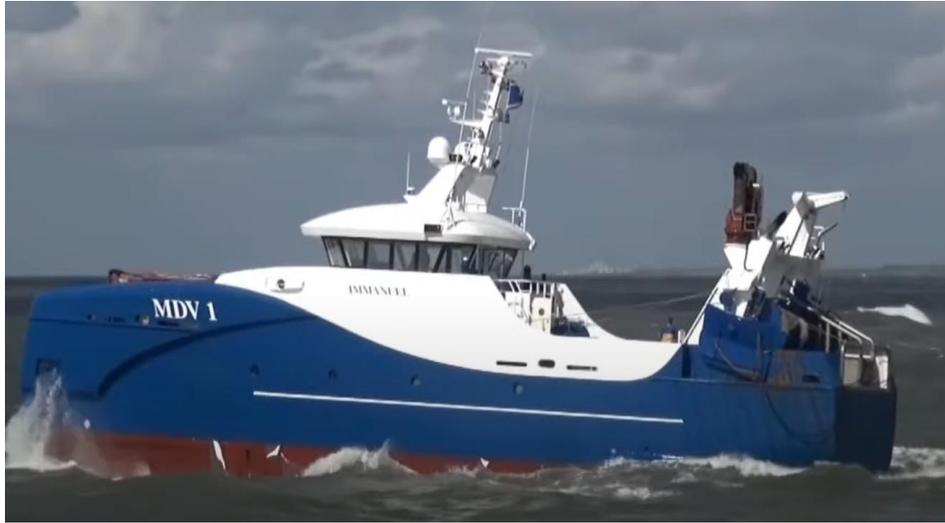
The **special shape** of the ship and the **diesel electric propulsion** provide **60% fuel and CO<sub>2</sub> savings** compared to comparable fishing vessels.
