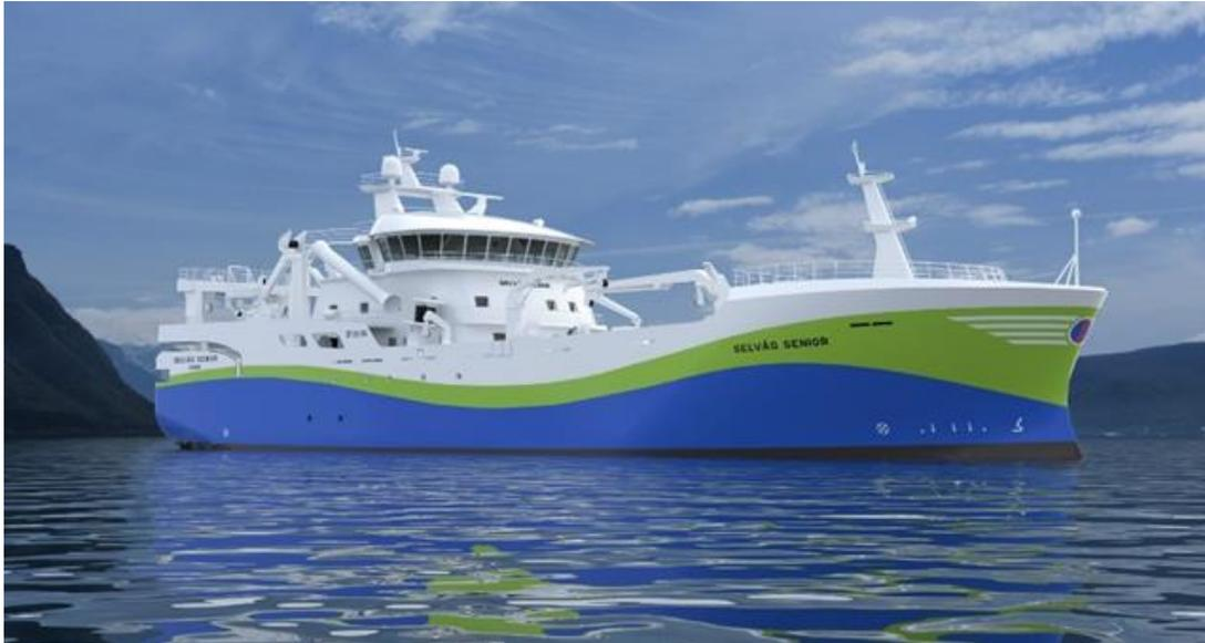
This 70m Norwegian longliner will have two **185-kW hydrogen fuel cells** and a **2,000-kWh battery bank**, as well as conventional diesel engines.
