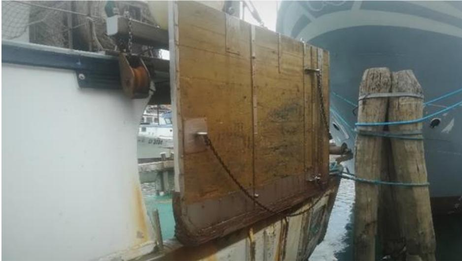
Some now use **otter doors with a metal frame and wood panels**. The lighter equipment **reduces seabed friction and fuel consumption**.
