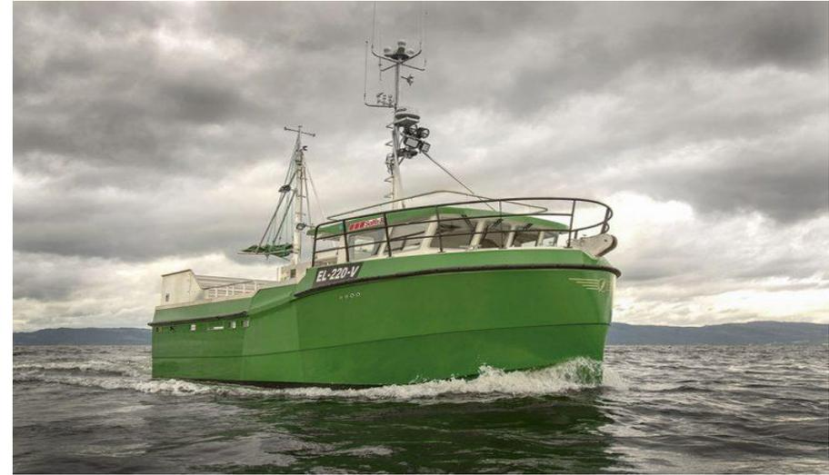
Equipped with **two battery packs of 195kWh** plus **500-litre diesel engine**. Diesel is used to and from the fishing grounds, then electric for fishing, loading and unloading.
